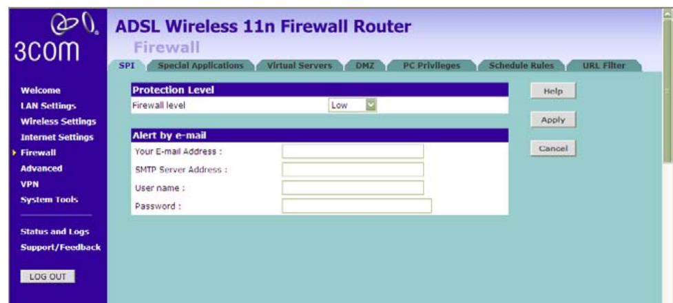
Figure 69 Low and Medium Level Firewall Protection Screen
