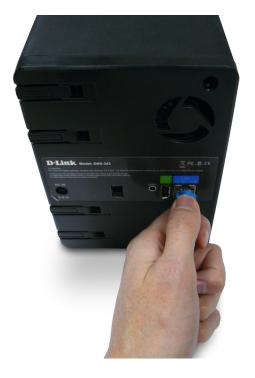
6. Connect the supplied power adapter to the power receptacle.
