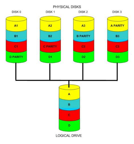
The DNS-343 supports the following configuration types: **Standard**, where each drive is a unique volume, **JBOD**, which combines both drives in a linear fashion to create one volume, **RAID 1** and **RAID 5** with a Basic Configuration and a combination of RAID 0/JBOD, RAID 1/JBOD and RAID 5/JBOD for Custom Configuration.
