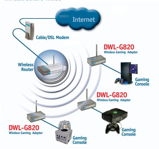
This example illustrates an **Infrastructure** setup. To connect the DWL-G820 to a wireless network with a wireless router or access point, please refer to the printed Quick Installation Guide included with the product. Web configuration is required to connect the DWL-G820.
