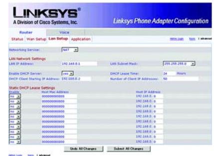
Figure 6-6: Router - LAN Setup Screen
