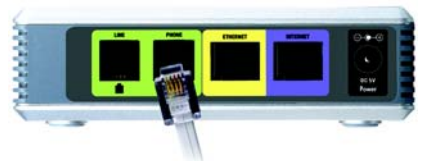
Figure 4-2: Connect a Telephone
