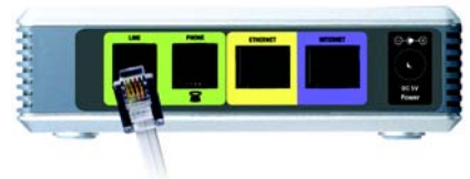
Figure 4-1: Connect to the Telephone Wall Jack
