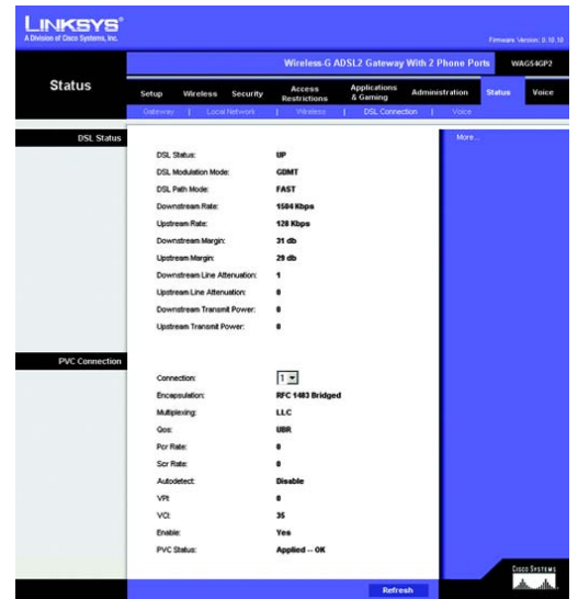
Figure 4-54: Status Tab - DSL Connection
