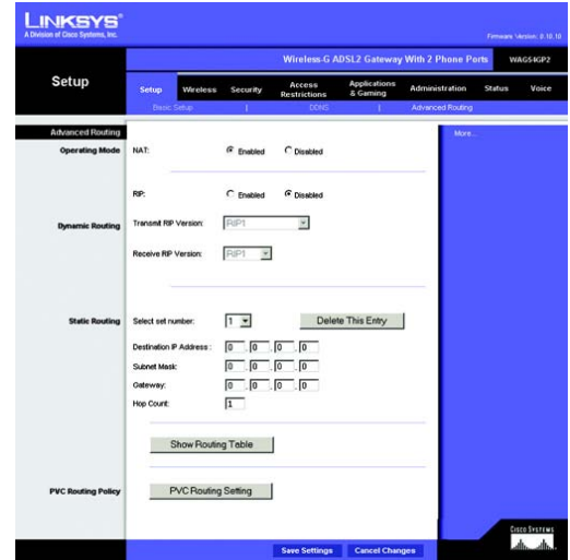
Figure 4-13: Setup Tab - Advanced Routing
