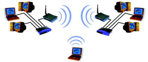
Figure 2-3: Network Using Wireless Bridging
