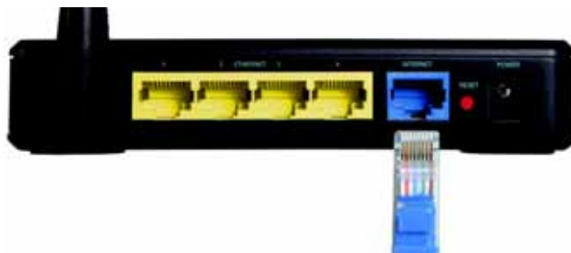
Figure 4-5: Connecting Another Router
