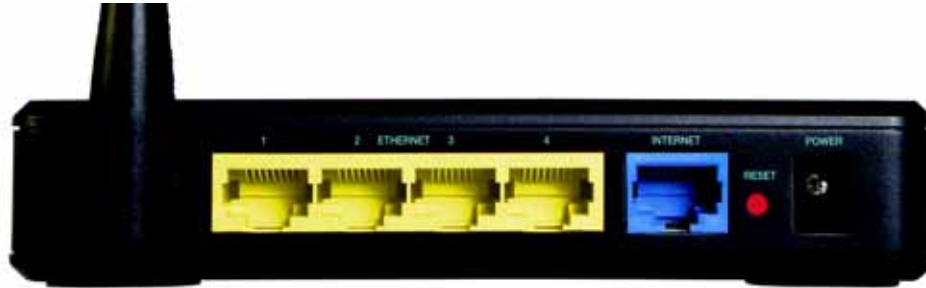
Figure 3-1: The Router's Back Panel
