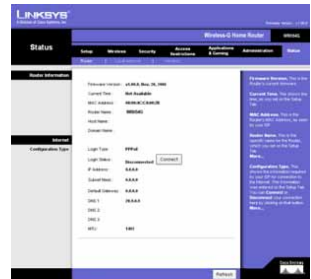
Figure 5-51: Status Tab - Router
