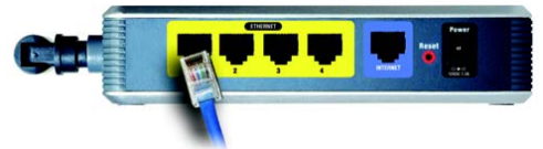
Figure 4-1: Connect a PC
