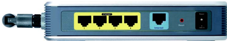
Figure 3-1: The Router's Side Panel
