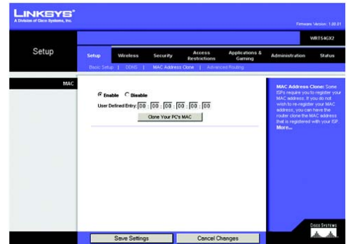
Figure 5-13: Setup Tab - MAC Address Clone
