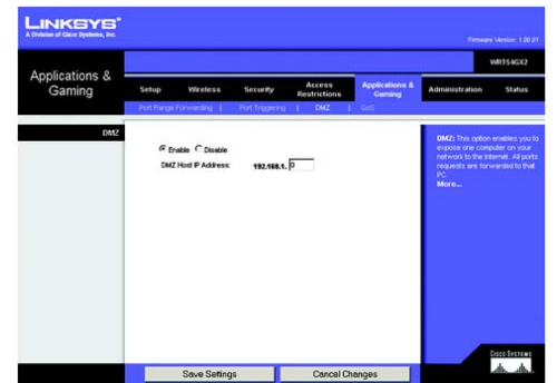
Figure 5-31: Applications and Gaming Tab - DMZ
