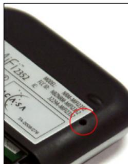
3. Insert a paper clip into the hole and hold the button down for **three seconds** until the LED goes out. The LED color will vary depending on the status of the device when you reset it.
