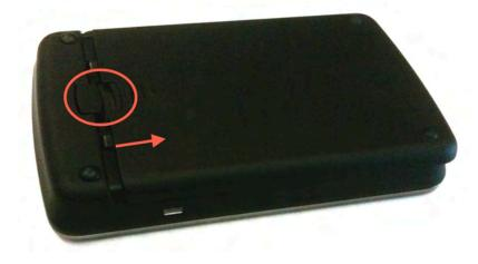
**2** Insert your fingernail into the battery removal divot and lift the battery out of the battery compartment.
