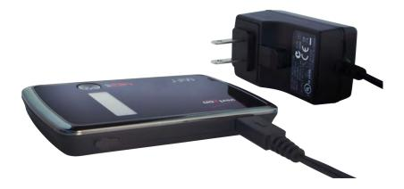
**IMPORTANT** When connecting the MiFi 4510L to your computer, it is recommended that a good quality shielded USB cable that is equal to or less than  $1 \text{ m} (\sim 3'3")$  in length be used.
