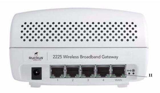
Figure 10—Rear View of the MM2225-NG with four LAN ports and one WAN port
