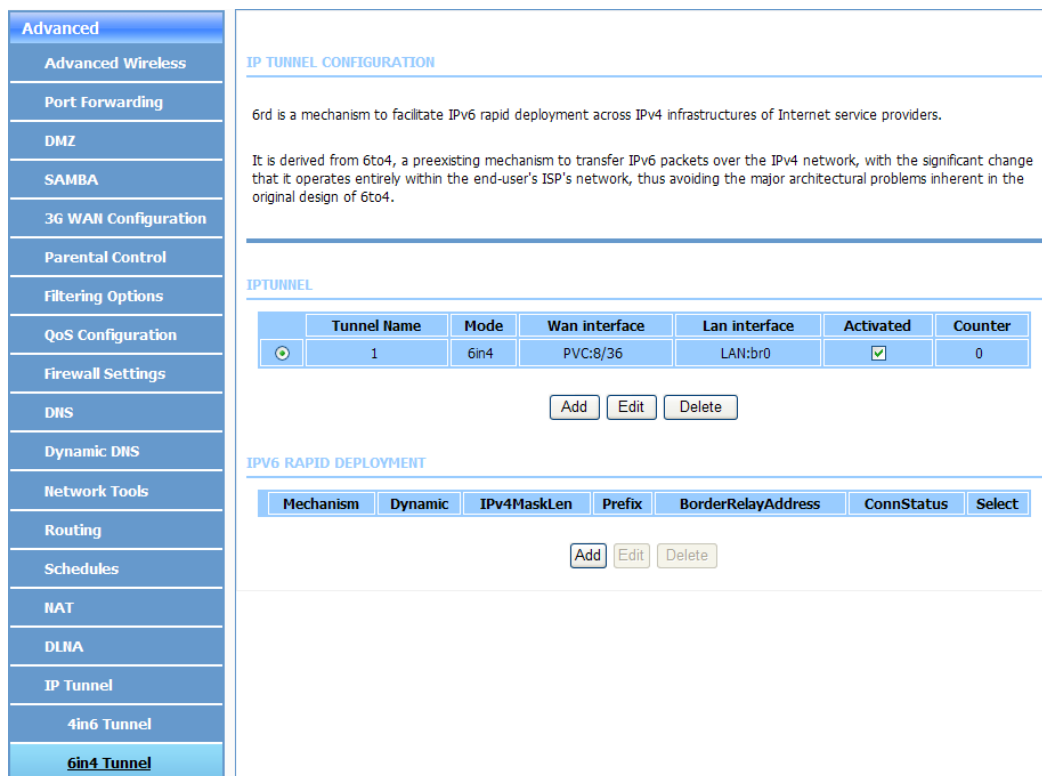
Figure 4-61 IP TUNNEL CONFIGURATION Page
