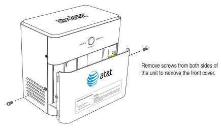
Figure 11: Power Supply Unit Cover Removal
