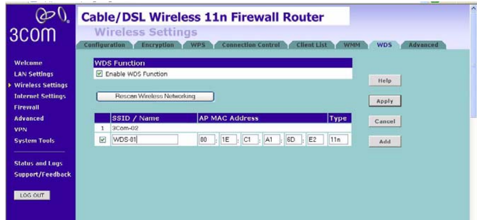
Figure 52 First Router add WDS Screen
