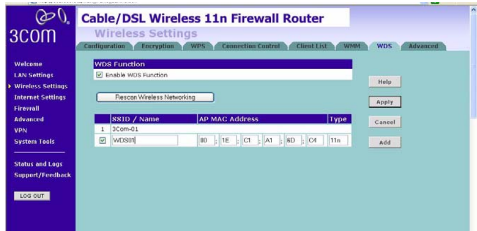
Figure 53 Second Router add WDS Screen
