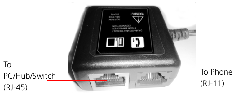
Figure 2-10: Data Equipment and Telephone Ports
