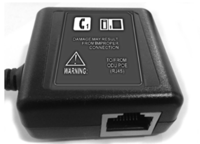
Figure 2-9: IDU-ODU PoE port ("TO/FROM ODU PoE (RJ45)")
