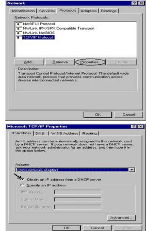
**3.**Select the **Obtain an IP address from a DHCP server** radio button and click **OK**.
