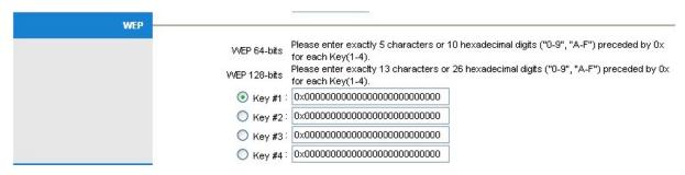
Key 1 to Key 4: Enter the key to encrypt wireless data. To allow encrypted data transmission, the WEP Encryption Key values on all wireless stations must be the same as the router. There are four keys for your selection. The input format is in HEX style, 5 and 13 HEX codes are required for 64-bitWEP and 128-bitWEP respectively.
