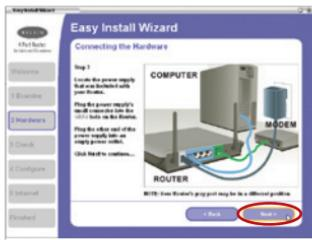
**2.3** This step instructs you to locate the power supply that is included with your Router. Plug the power supply's small connector into the power port on the Router. Plug the power supply into an empty power outlet. Click “Next” to continue.
