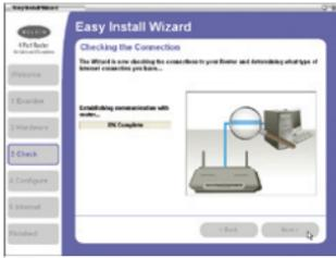
**3.1** Once you have completed connecting the Router, the Wizard will check the connection to the Router and then go on to determine what type of Internet connection you have.
