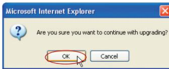
5. You will see one more message. This message tells you that the Router may not respond for as long as one minute as the firmware is loaded into the Router and the Router is rebooted. Click “OK”.
