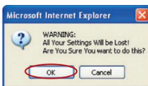
3. The following message will appear. Restoring the defaults includes restarting the Router. It can take up to 25 seconds. It is important not to turn the power to the Router off during the restart.
