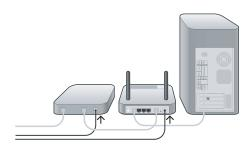
Plug in your modem's power cord. Wait 60 seconds for the modem to start up. Plug the Router's power supply into the black port on the back. Plug the other end into the wall outlet.
