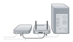
Find your new networking cable (included in the box with your Router) and connect it to the yellow port on the back of the Router. Connect the other end to your modem, in the port that's now free.
