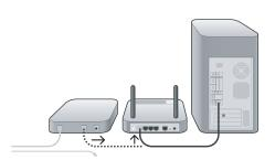
В. Locate the networking cable that connects your modem and computer. Unplug that cable from your modem, and plug it into any gray port on the back of the Router.
