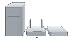
Wait 20 seconds for the Router to start up. Look at the display on the front of the Router. Make sure the "Wired" and "Router" icons are lit up in blue. If they are not, recheck your connections.
