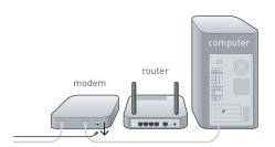
Unplug your modem's power cord. Put the Router next to the modem. Raise the Router's antennas.
