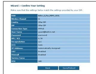
3.3 Now you have configured your modem router. Click on the OK button to apply the settings. After a period of about 2 minutes the connection with the Internet Service Provider will be established.
