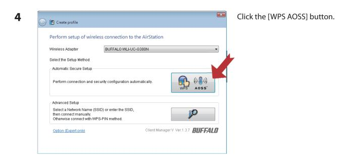
Follow any instructions displayed on the screen. When the Security LED on the front of the AirStation stops flashing and is lit steadily, the connection is complete.
