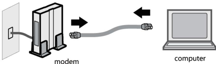
**3** Plug one end of the LAN cable into your modem and the other end to the AirStation's Internet (WAN) port. Turn on the modem.
