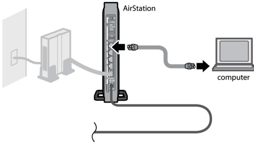
**Note:** If the power does not turn on when the AC adapter is connected, press the Power button on the rear of the AirStation.
