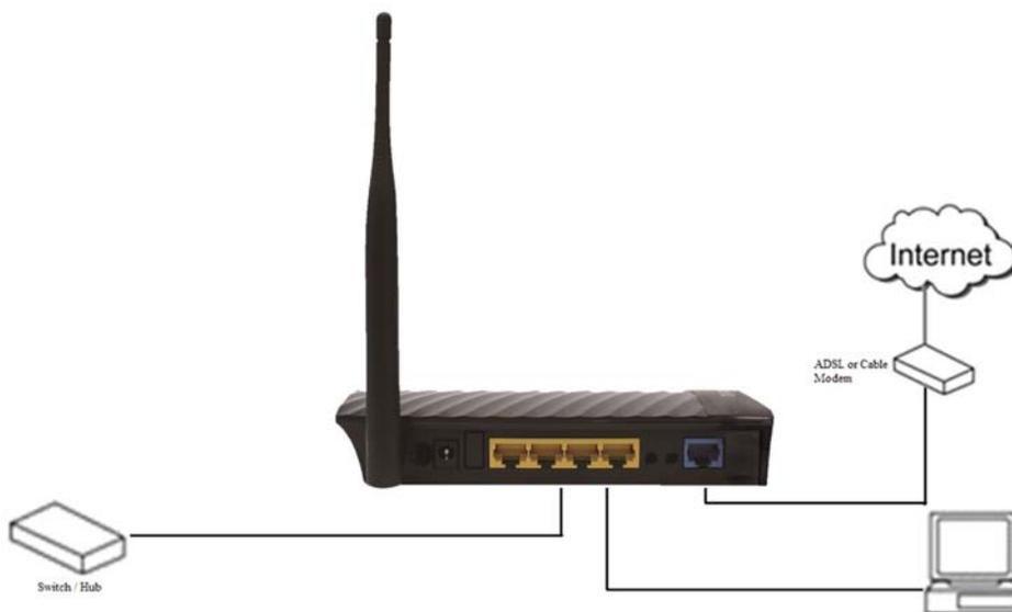
3. Connect the power adapter (5V DC / 1A) to the wall socket, and then connect it to the '**P**ower' socket of the router.
