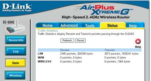
The screen above displays the Traffic Statistics. Here you can view the amount of packets that pass through the DI-624S on the WAN, LAN, and Wireless interfaces. The traffic counter will reset if the device is rebooted.
