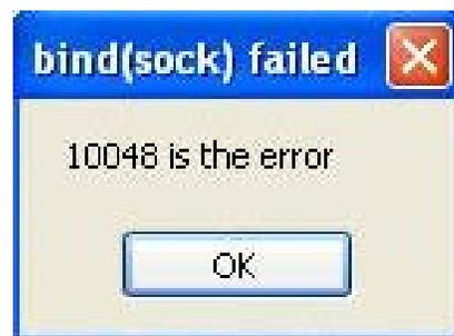
This Windows error will occur if the Internet Camera is connected to a computer that is not properly configured with a valid IP address. Turn off DHCP from the Network Settings in Windows and configure the computer with a valid IP address or connect the camera to a router with DHCP enabled.
