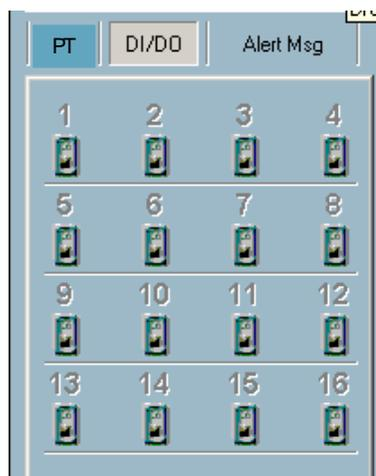
Clicking on the “DI/DO” button shown below, you can switch to the DI/DO controls. The color of the channel number indicates the status of the camera’s DI (Digital Input). You can click the “Switch button” to change the HI/LOW state of the DO (Digital Output). With these features, you can monitor the remote sensor input from DI and also trigger the camera by DO switch.
