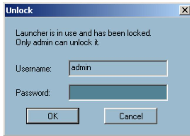
The input area of the dialog will be grayed (disabled) for 60 seconds after 3 consecutive failures.
