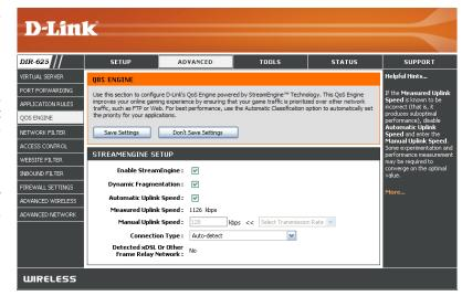
Manual Uplink The speed at which data can be transferred from the router to your ISP. This is determined by your ISP. ISP's often speed as **Speed:** a download/upload pair. For example, 1.5Mbits/284Kbits. Using this example, you would enter 284. Alternatively you can test your uplink speed with a service such as www.dslreports.com.
