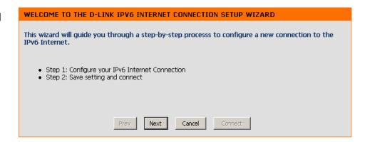
The router will try to detect whether its possible to obtain the IPv6 Internet connection type automatically. If this succeeds then the user will be guided through the input of the appropriate parameters for the connection type found.
