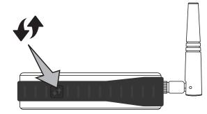
**Step 2** - Within 2 minutes, press the WPS button on your wireless client (or launch the software utility and start the WPS process).
