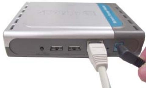
Attach your USB drive(s) to the USB port(s) on the rear panel of the DNS-120.
