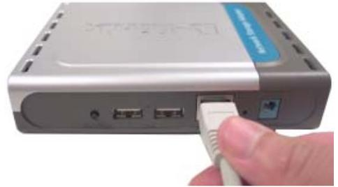
Attach the other end of the provided Ethernet cable to an available Ethernet port on your router or switch.
