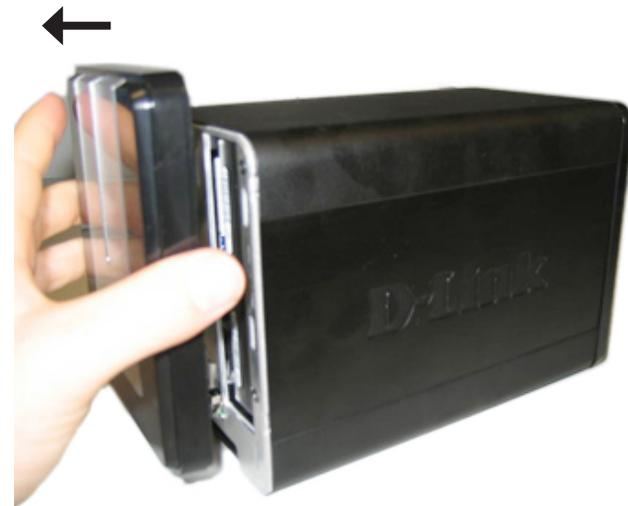
3. Insert a 3.5" SATA hard drive into each available drive bay. Make sure to align the drive connectors to the endpoints in the DNS-323. Gently push the drive in until it connects.
