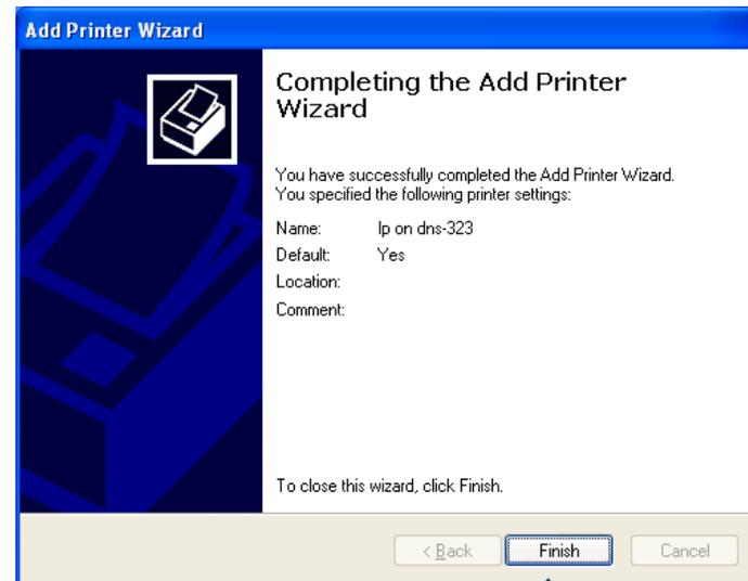
The wizard will install the printer drivers, and return a completion screen. Click **Finish**.
