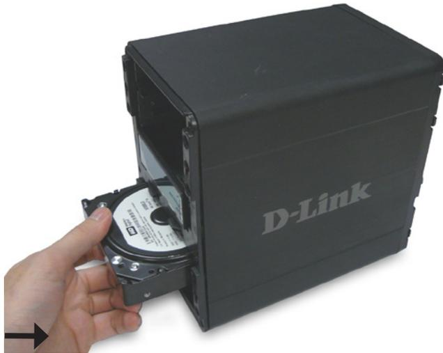
3. Insert a 3.5" SATA hard drive into each available drive bay. Make sure to align the drive connectors to the SATA connectors on the bottom edge inside the drive bay of the DNS-343. Gently push the drive in until it connects. When a drive is inserted properly, you will feel it "seat" into the connector. Some hard drives that are thin or oddly shaped may need to be guided carefully into position.
