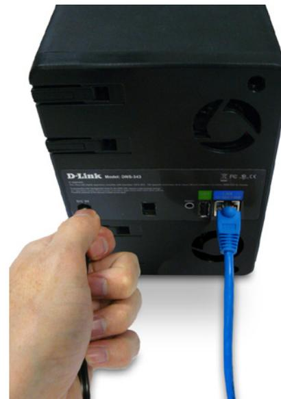
6. Connect the supplied power adapter to the power receptacle.
