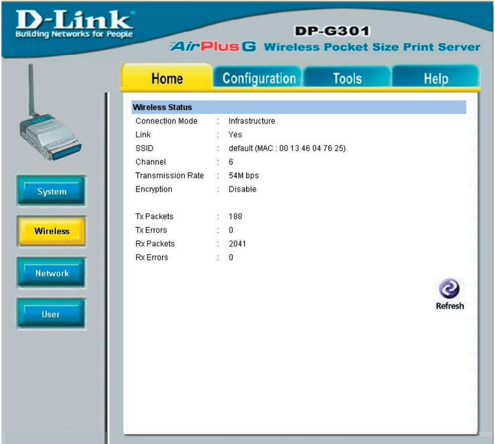
The screenshot displays the web configuration interface for the D-Link DP-G301 AirPlus G Wireless Pocket Size Print Server. The interface includes a navigation menu on the left with buttons for System, Wireless, Network, and User. The main content area shows the 'Wireless Status' section with the following information:
