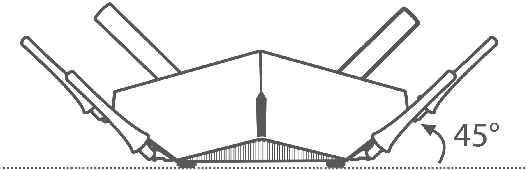
NOTE: Attach the antennas to the router before powering it on.
