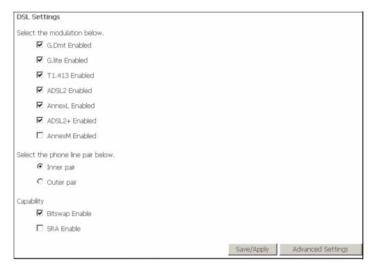
Select the desired DSL test mode and then click the **Apply** button.
