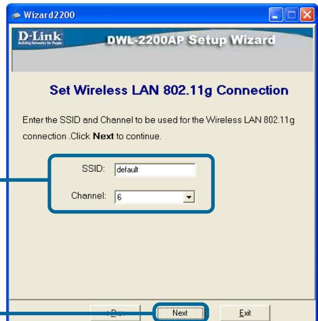
Enter the **SSID** and the **Channel** for the network.
