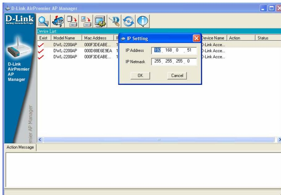
Select the AP that you want to assign an IP address and click the IP button. Enter the IP Address and IP Netmask for the selected device and click OK.
