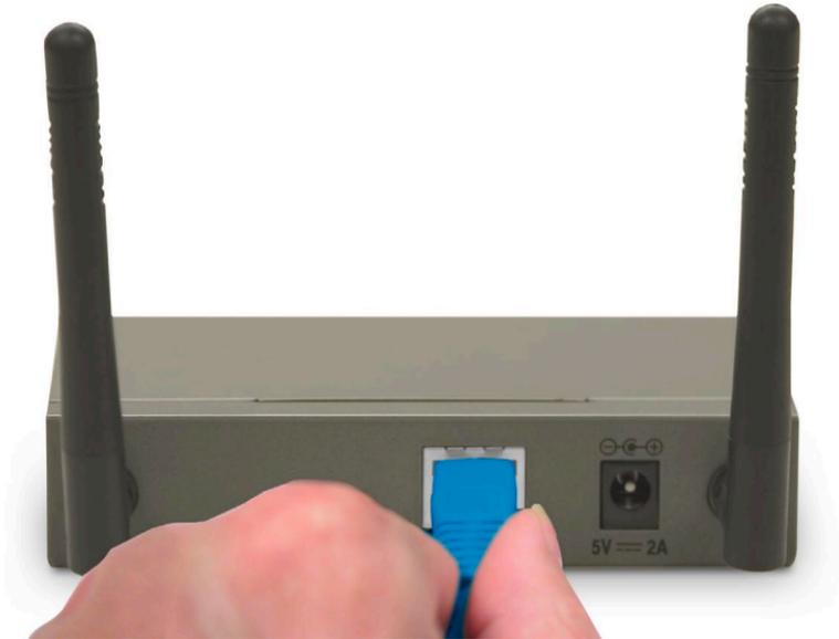
Insert the supplied Ethernet cable to the DWL-3150 and connect the other end to your computer or network.
