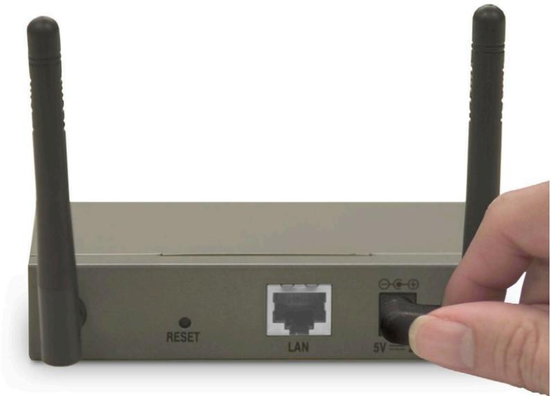
Insert the supplied power supply to the DWL-3150 and plug the other end into an outlet or power strip. The unit will power on.
