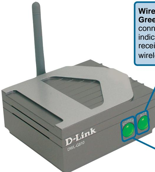
**Wireless Link/Act** – a steady **Green** light indicates a wireless connection. A blinking light indicates that the DWL-G810 is receiving/transmitting from/to the wireless network.
