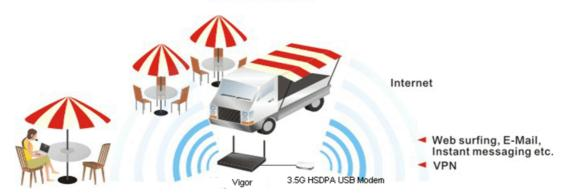
After connecting into the router, 3G USB Modem will be regarded as the second WAN port. However, the original Ethernet WAN1 still can be used and Load-Balance can be done in the router. Besides, 3G USB Modem in WAN2 also can be used as backup device. Therefore, when WAN1 is not available, the router will use 3.5G for supporting automatically. The
