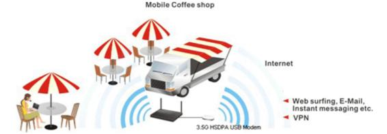
After connecting into the router, 3G USB Modem will be regarded as the second WAN port. However, the original Ethernet WAN1 still can be used and Load-Balance can be done in the router. Besides, 3G USB Modem also can be used as backup device. Therefore, when WAN1 is not available, the router will use 3.5G for supporting automatically. The supported 3G USB
