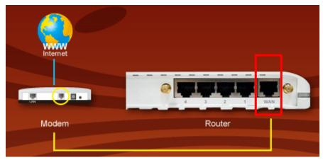
Connect all your computers, network devices (network-enabled consumer devices other than computers, like game console, or switch / hub) to the LAN (1-4) port of the router.
