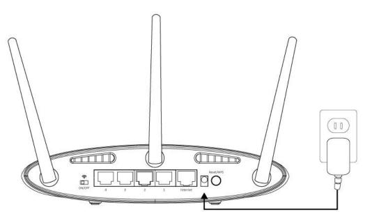
2. Ensure that the Wi-Fi On/Off switch is set to on and that three LEDs (power, 2.4GHz & 5GHz Wi-Fi) display on.
