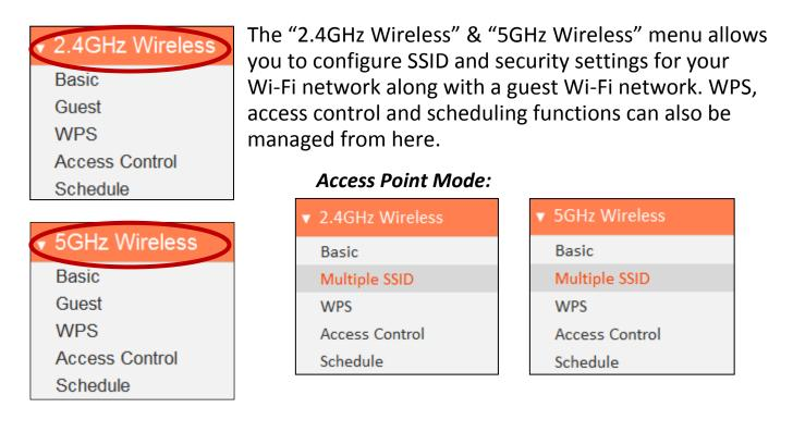
In Access Point mode, the "Guest" feature in the menu is replaced by "Multiple SSID".
