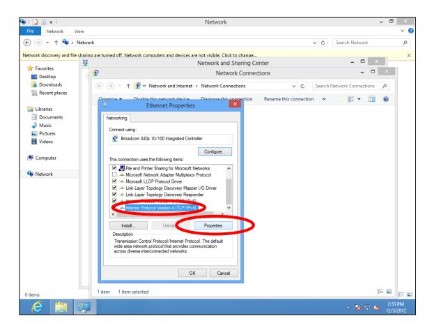
**7.** Select "Use the following IP address" and "Use the following DNS server addresses", then input the following values:
