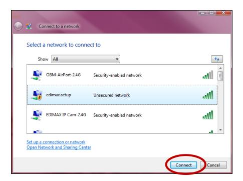
**3.** After correctly entering your password, you will be successfully connected to the BR-6208AC's wireless network.
