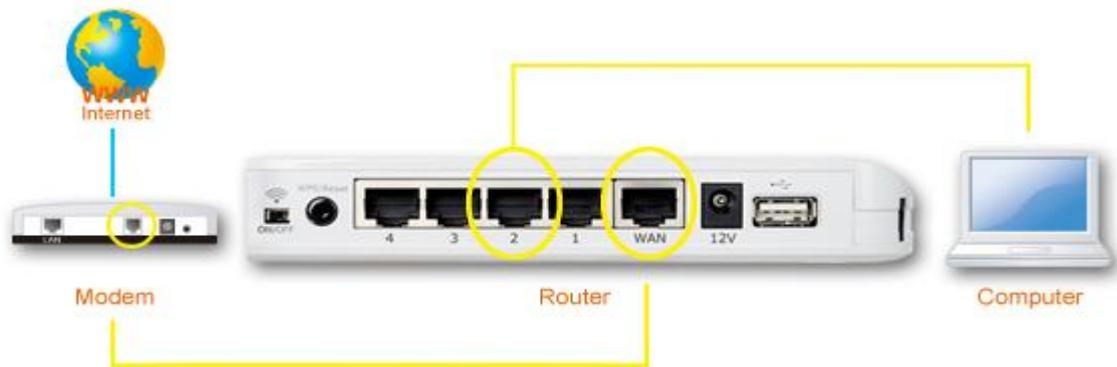
Before using the BR-6478AC, please make sure your computer is set to use a **dynamic IP address**. This means your computer can obtain an IP address automatically from a DHCP server. Please refer to instructions appropriate for your operating system.
