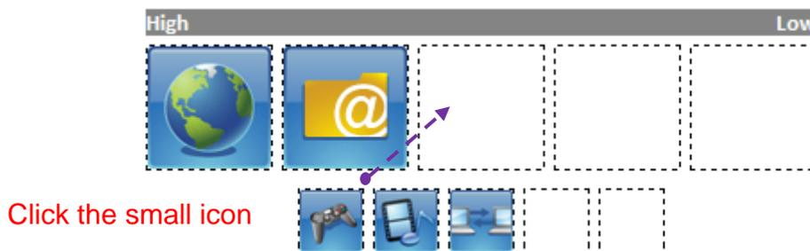
Check the box "Enable iQoS" to enable this feature. Specify the total upload and download bandwidth and then arrange the network application icons in priority order. Network applications are grouped into the following five categories:
