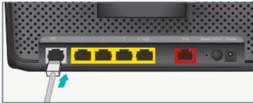
**1.1** Plug the other end of the grey broadband cable into the DSL/fibre port on your router.
