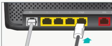
Plug one end of the black Ethernet cable into any of the yellow Ethernet sockets on the back of your EE router.
