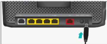
**1.3** Plug the power cable into the router.
