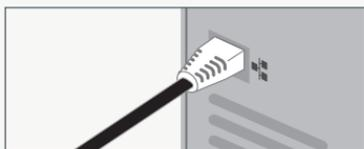
Plug the other end into the Ethernet socket on your device.
