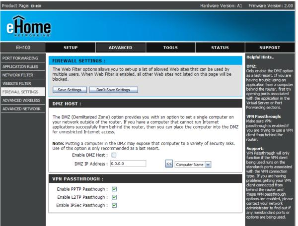
Enable DMZ Host: Check this box to enable DMZ.
