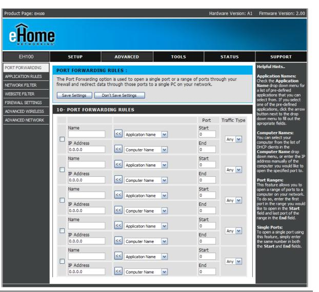
To create a Port Forwarding rule, check the box to enable the rule, and fill in the required configuration fields.
