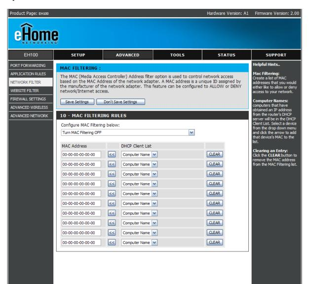
To create an Network Filter rule, check the box to enable the rule, and fill in the required configuration fields.
