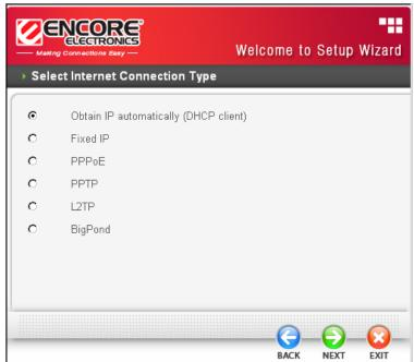
If the user has enabled DHCP server, choose "Obtain IP automatically (DHCP client)" to have the WLAN Router assign IP addresses automatically.
