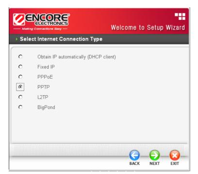
If connected to the Internet using a PPTP xDSL connection, enter your IP, Subnet Mask, Gateway, Server IP, PPTP Account and PPTP Password.
