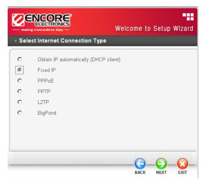
If the Internet Service Provider (ISP) assigns a fixed IP address, choose this option and enter the assigned WAN IP Address, WAN Subnet Mask, WAN Gateway Address and DNS Server Addresses for the WLAN Router.
