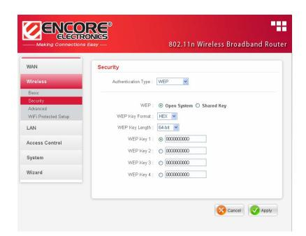
**WEP:** Open System and Shared Key requires the user to set a WEP key to exchange data with other wireless clients that have the same WEP key.
