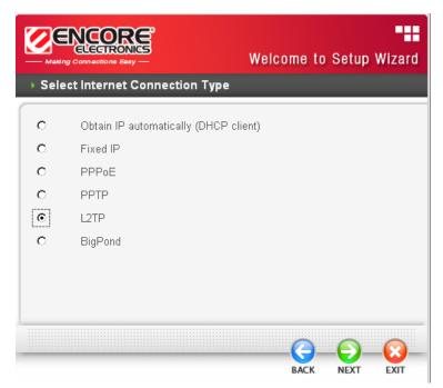
If connected to the Internet using a L2TP (Dial-up xDSL) connection and the ISP provides a Server IP, Account and Password information, choose this option and enter the required information.
