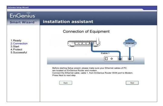
Check the MODEM and ESR-9752 connection. It should be as shown below.
