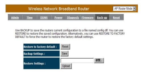
Backup Settings: This can save the Broadband router current configuration to a file named "config.bin" on your PC. You can also use the <Upload> button to restore the saved configuration to the Broadband router. Alternatively, you can use the "Restore to Factory Defaults" tool to force the Broadband router to perform a power reset and restore the original factory settings.
