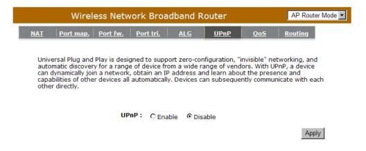
**Enable/Disable UPnP:** You can enable or Disable the UPnP feature here. After you enable the UPnP feature, all client systems that support UPnP, like Windows XP, can discover this router automatically and access the Internet through this router without having to configure anything. The NAT Traversal function provided by UPnP can let applications that support UPnP connect to the internet without having to configure the virtual server sections.
