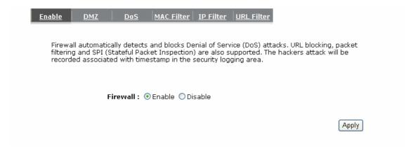
Note: To enable the Firewall settings select Enable and click Apply
