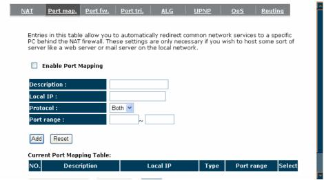
**Enable Port Mapping:** Enable or disable port mapping function.
