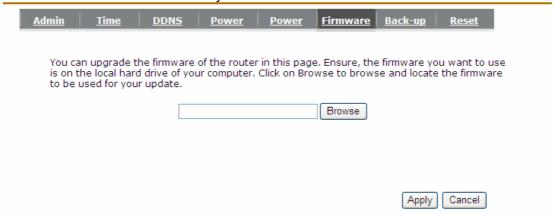
Once you've selected the new firmware file, click **Apply**> at the bottom of the screen to start the upgrade process
