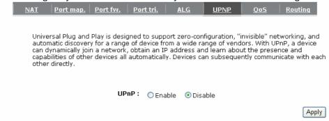
**Enable/Disable UPnP:** You can enable or Disable the UPnP feature here. After you enable the UPnP feature, all client systems that support UPnP, like Windows XP, can discover this router automatically and access the Internet through this router without having to configure anything. The NAT Traversal function provided by UPnP can let applications that support UPnP connect to the internet without having to configure the virtual server sections.
