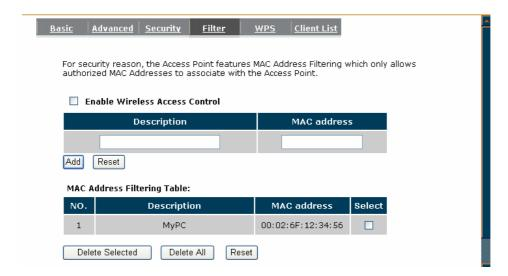
Enable wireless access control: Enable the wireless access control function
