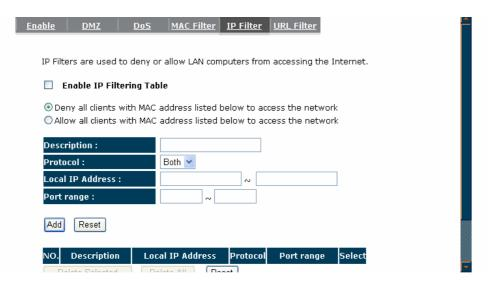
**Enable IP Filtering:** Check to enable or disable IP Filtering.
