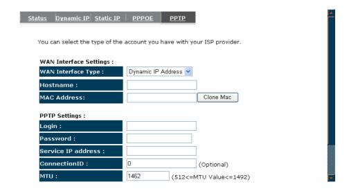
PPTP allows the secure connection over the Internet by simply dialing in a local point provided by your ISP provider. The following screen allows client PCs to establish a normal PPTP session and provides hassle-free configuration of the PPTP client on each client PC.
