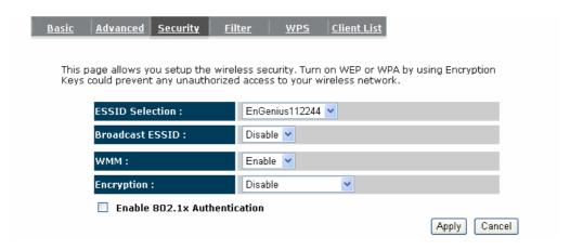
**ESSID Selection:** This broadband router support multiple ESSID, you could select and set up the wanted ESSID.
