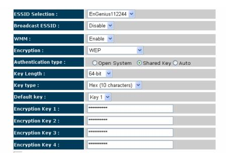
Authentication Type: There are two authentication types: "Open System" and "Shared Key". When you select "Open System", wireless stations can associate with this wireless router without WEP encryption. When you select "Shared Key", you should also setup a WEP key in the "Encryption" page. After this has been done, make sure the wireless clients that you want to connect to the device are also setup with the same encryption key.
