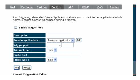
**Enable Trigger Port:** Enable or disable the Port Trigger function.
