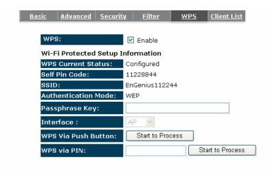
WPS: Check the box to enable WPS function and uncheck it to disable the WPS function.
