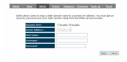
Enable/Disable DDNS: Enable or disable the DDNS function of this router
