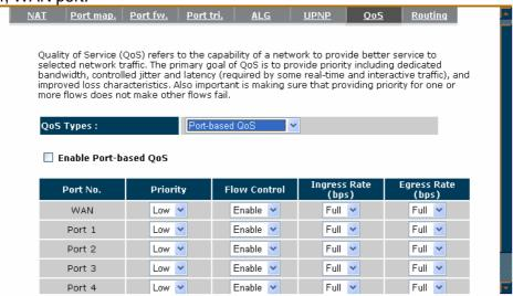
**Enable Port-based QoS:** Check this to enable port-based QoS functionality for the LAN/WAN port. You can also uncheck to disable.
