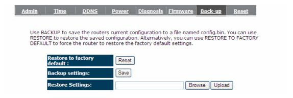
**Backup Settings:** This can save the Broadband router current configuration to a file named "config.bin" on your PC. You can also use the <Upload> button to restore the saved configuration to the Broadband router. Alternatively, you can use the "Restore to Factory Defaults" tool to force the Broadband router to perform a power reset and restore the original factory settings.
