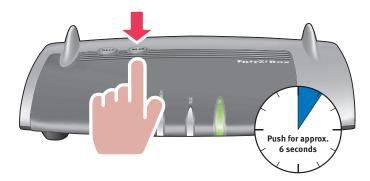
As soon as the "WLAN" LED begins flashing, enable the WPS function on the other WLAN device, either by pressing a button or in the device's user interface (depending on the device). Activation must be started within two minutes.
