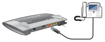
Connecting an IP telephone to the network port of the FRITZ!Box
