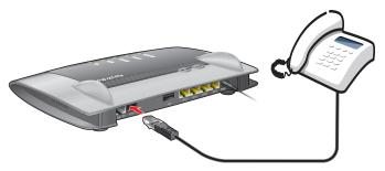
Connecting an analog telephone with an RJ11 plug
