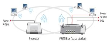
WDS: Expanding the WLAN range using a WDS repeater
