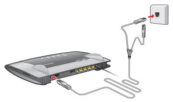
Connecting using DSL/telephone cable
