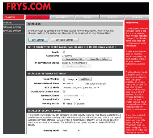
Wireless Channel: Indicates the channel setting for the FR-300RTR. By default the channel is set to 6. The Channel can be changed to fit the channel setting for an existing wireless network or to customize the wireless network. If you enable **Auto Channel Scan**, this option will be greyed out.
