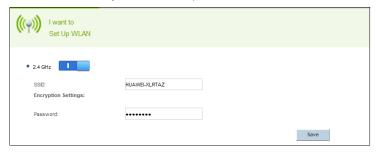
To obtain the default SSID and key, check the label on the rear panel. To better secure your WLAN, promptly change the SSID and key.
