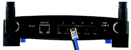
Figure 4-2: Connecting Your Network Devices
