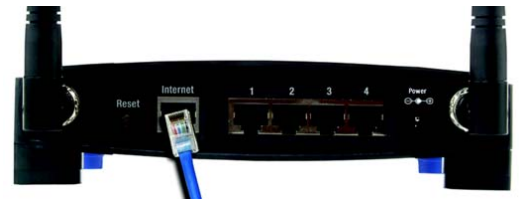
Figure 4-1: Connecting Your Internet Connection
