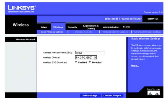
Figure 5-13: Wireless Tab - Basic Wireless Settings
