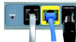
Figure 3-5: Connect to the Power Port
