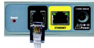
Figure 3-3: Connect to the LINE Port
