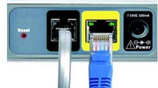
Figure 3-4: Connect to the Ethernet Port
